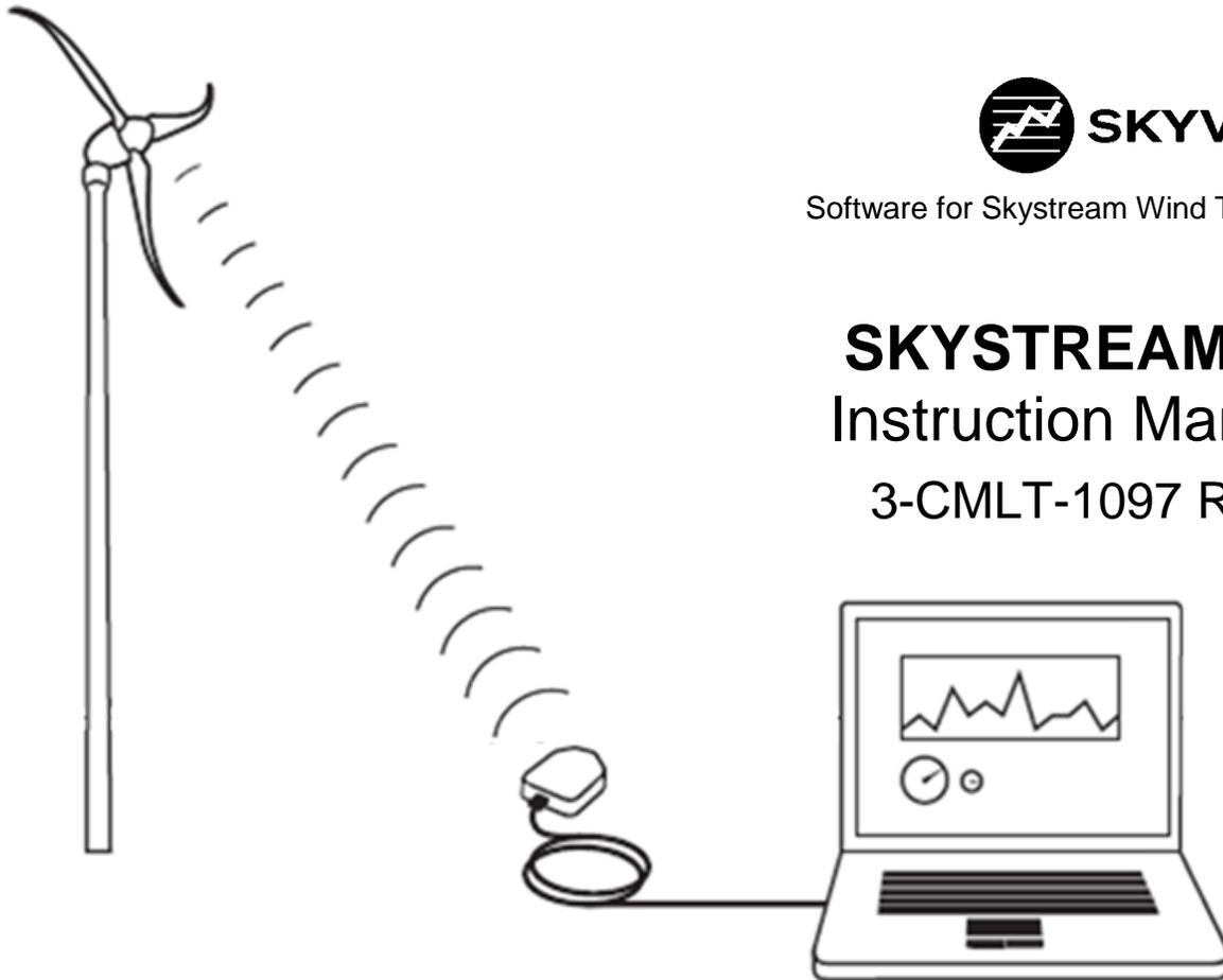
The Wireless PC Interface and Skyview 2.0 Software are compatible with Skystream 3.7 wind generators with installed 2.4 GHz communications packages and inverter firmware version 2.02 (and greater).
